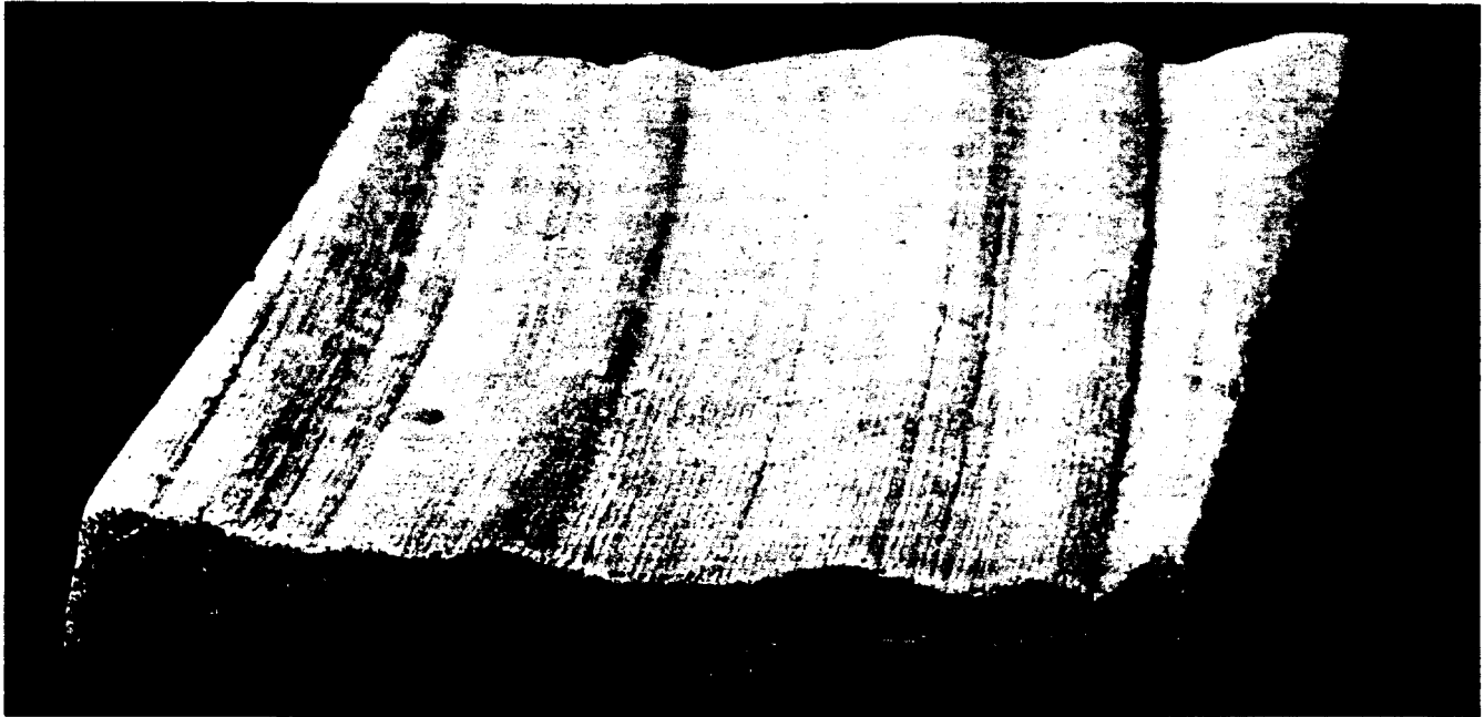
Fig. 4.4 Severe collapse in western red cedar
