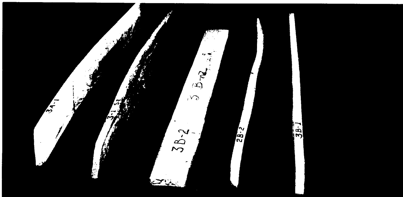
Fig. 4.3 Shrinkage defects in lumber, left to right: bow, combined bow and cup, unwarped, combined crook and kink, twist
