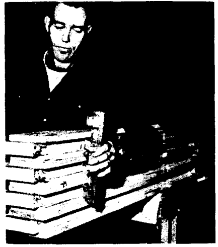
Jigs used to set T&G pattern in sides rides through press with stock. They keep stock away from electrodes, prevent slippage. Jigs are of plywood.
