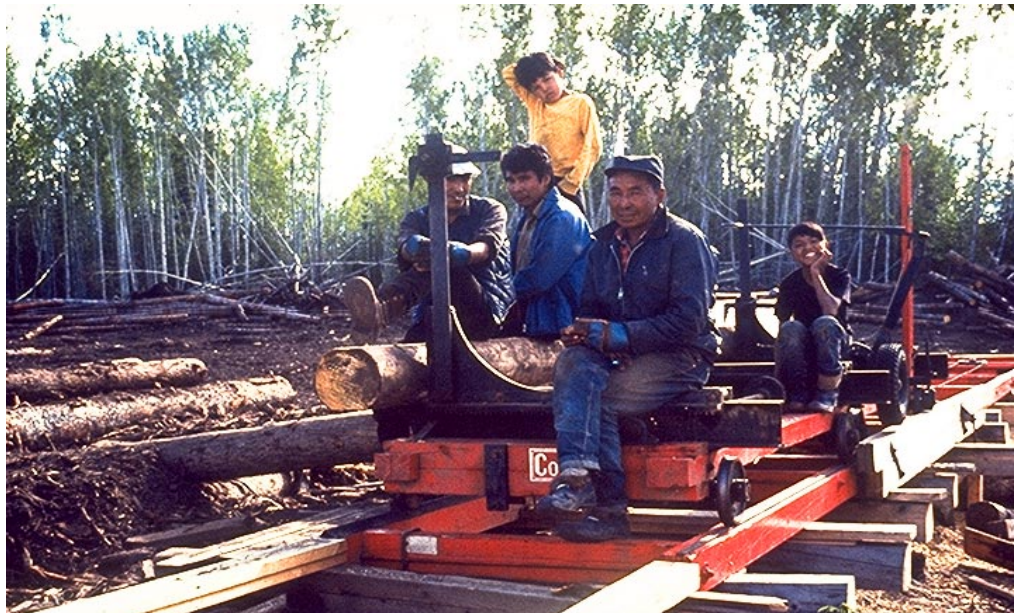
A small community sawmill for manufacturing lumber.
